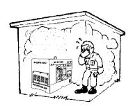
enclosed or narrow area where free flow of the air is restricted. If the air flow is restricted it will cause serious damage to the welder/generator engine and may cause injury to people. Remember the welder/generator's engine gives off DEADLY carbon monoxide gas.
